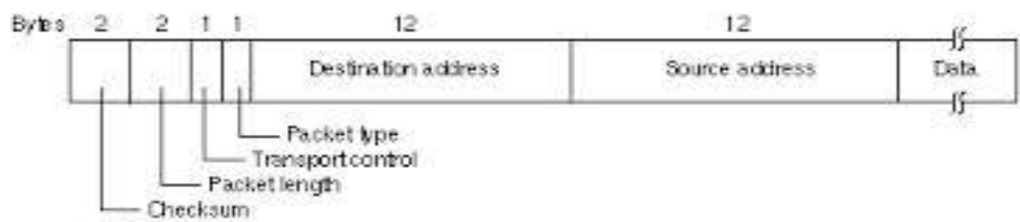
Fig. 2: A Novell NetWare IPX packet.
